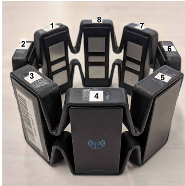
Figure 3.1: The Myo Armband showing the labels for each sensor. The IMU is located within Sensor 4.
