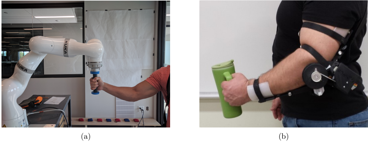
Figure 2.2: Example of robotic devices that can be used during upper limb rehabilitation. The KUKA robot, a serial robotic manipulator (a), and the WearME Brace [40], a wearable mechatronic device (b).
